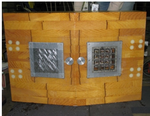
Figure 4-2: Photograph of instrumented wedge used in NSWCCD experiment.
